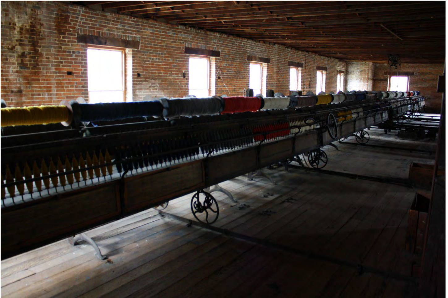
Photo 0028 MO_Clay County_Watkins Mill_0028 Watkins Mill, third floor, spinning jacks, camera facing northeast
