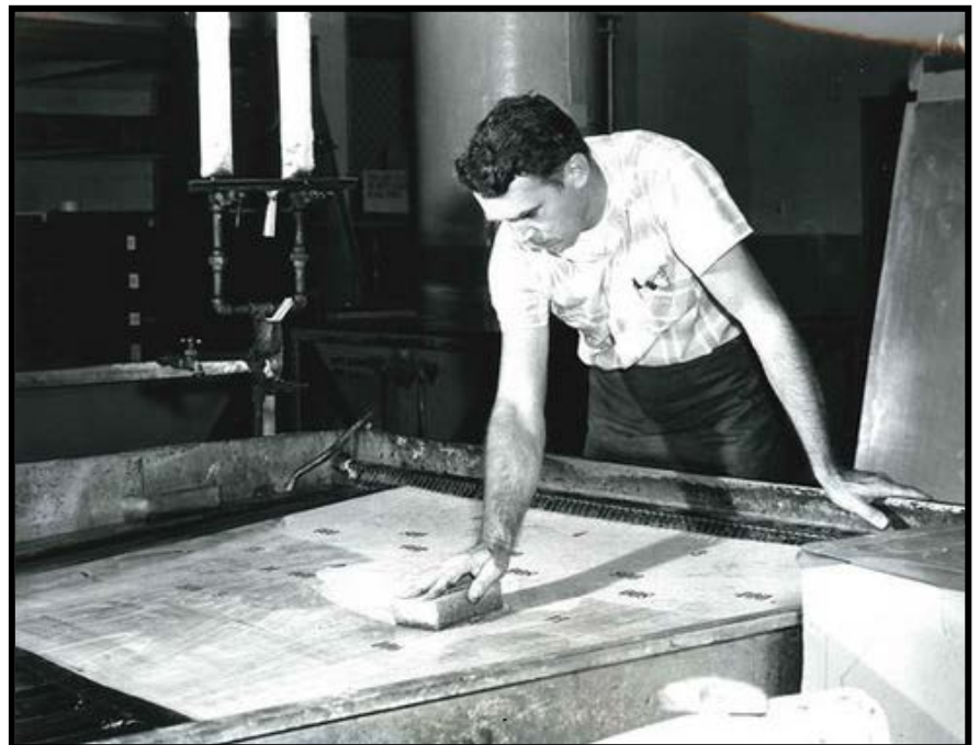
Figure 34: Employee at work on developing and cleaning color plates for charts at the building. Source: NGA St. Louis archives.
