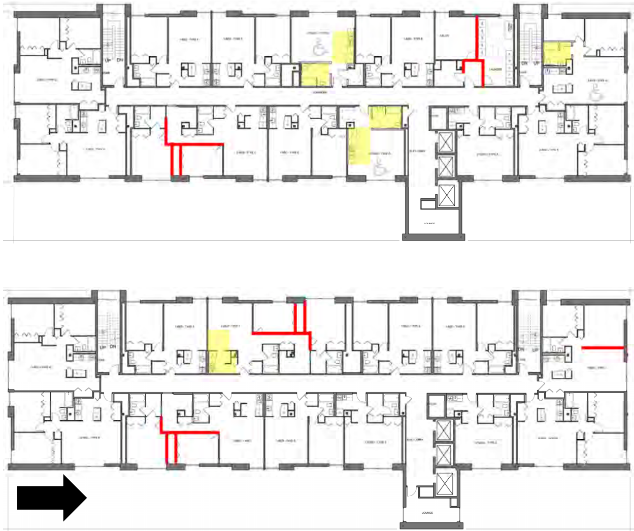
Figure 5. Excerpts of current second floor (top) and typical current upper floor configuration (bottom, seventh floor shown). New walls highlighted in red, reconfigured kitchens highlighted (Ebersoldt + Associates Architecture, “Heritage House,” (2023), A102-A103, plans from owner).
