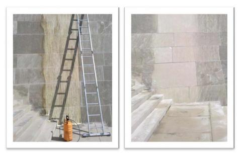
Left: Cleaning test on limestone with gentlest chemical cleaner available and lowpressure water rinsed. Right: After image of cleaning, no abrasives or highpressure water was used. Cleaner did not harm the stone. Kansas City, MO 2010.
